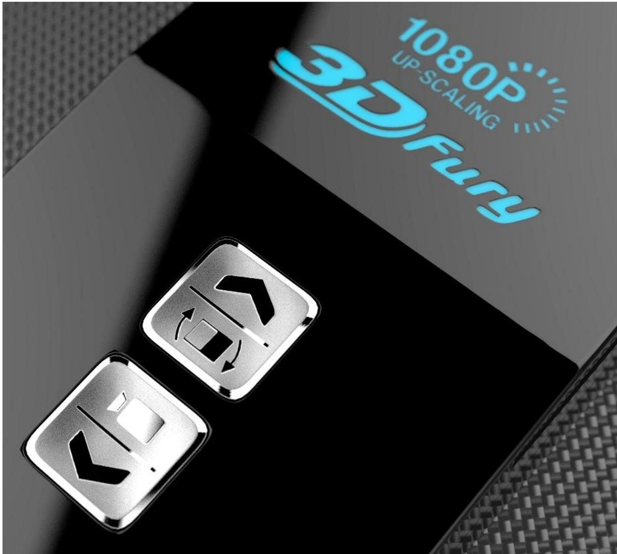
The HDfury4S logo will glow blue when in use. When the HDfury4S first receives an HDMI signal the logo will quickly turn on, then off, and then on permanently to indicate that the 4-letters handshake has been completed.
