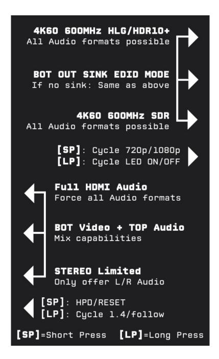
A sticker is available on the back of the unit to remind you the basic configuration options available from the physical button and slide switches.
