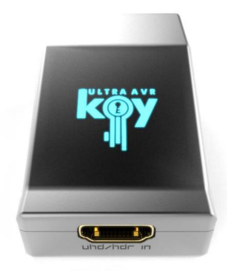
The AVR-Key logo will glow Blue when in use. When the AVR-Key first receives an HDMI signal the logo will quickly turn on, then off, and then on permanently to indicate that the HDCP handshake has been completed.
