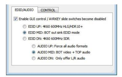
[Enable GUI Control]: Check this box to disable slide switch and set the unit configuration via GUI.
