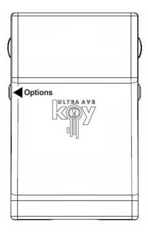
Options Button allows you to cycle audio stream output resolution and turn LOGO Led ON/OFF.
