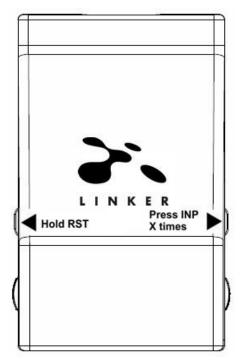
For users without access to GUI for Windows PC, we added a dual-button combo, when RESET is pressed down and INPUT is clicked the **CS** (Color Space) and **DC** (Deep Color) mode presets cycle between
