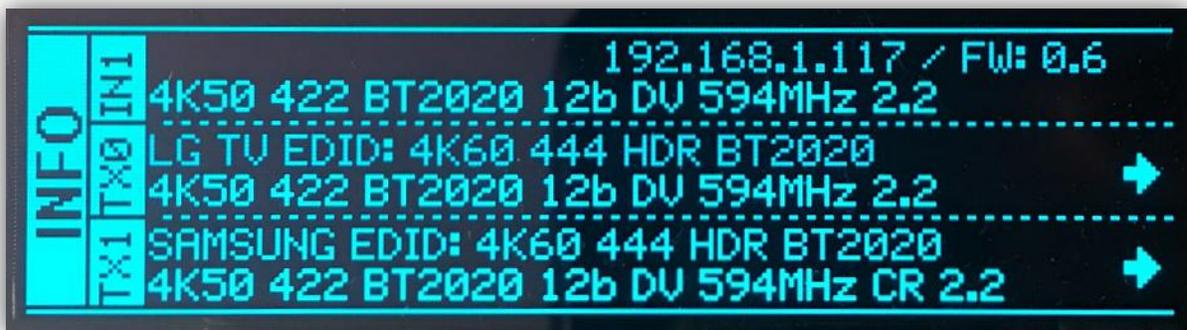
**[192.168.1.117]:** VRROOM IP address will be displayed here if LAN CONTROL RJ45 output is connected to your LAN/WAN router/switcher. mDNS and other way are available if you cycle OLED infopage.
